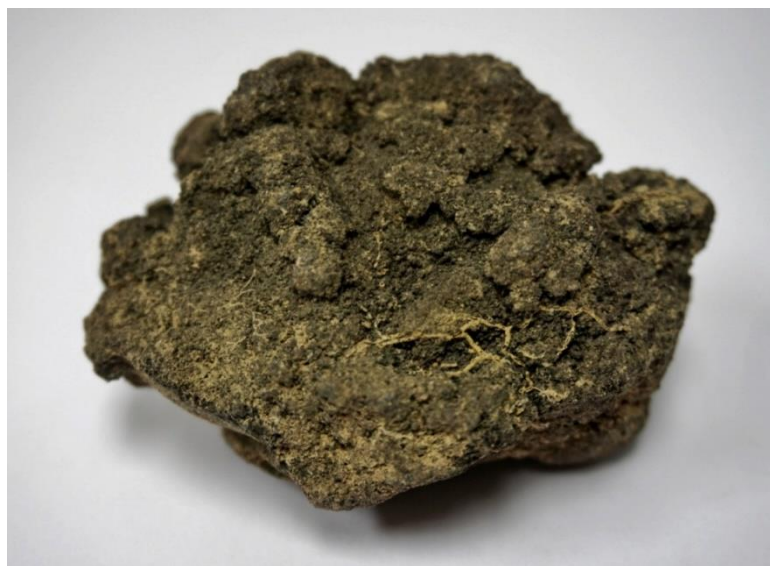
Figure 1.2 A polymetallic nodule, also called a manganese nodule or ferromanganese nodule. Image credit: K. McQuaid.
