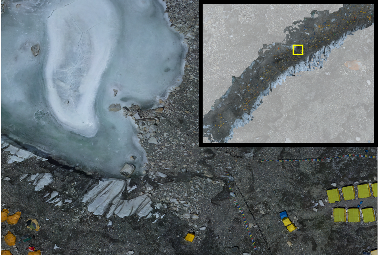
Figure 2. High-resolution 3D scans of basecamp show many instances of tents erected near melt pools as seen in this image. These melt pools hint at the amount of liquid water that may be on top of and beneath the glacier surface, creating significant risks to basecamp through possible surface collapse, supraglacial flooding and glacial outburst flooding.
