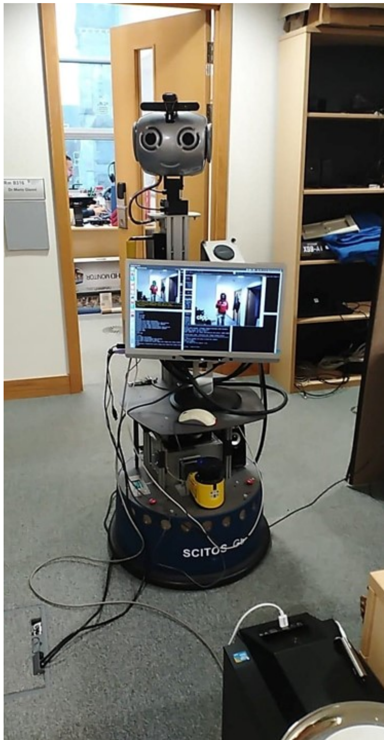
Figure 2.4: Pre-experimental setup of the robot with face tracking already implemented. For the data gathering, the console was occluded and a simple word representing an action would be shown on the screen, together with pre-recorded synthetic audio instructions. Initially the plan was to gather a dataset with multiple subjects, but in the end the set was simplified to a single subject, me.
