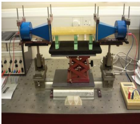
Fig. 3 Microwave input/output experimental coupling apparatus.
