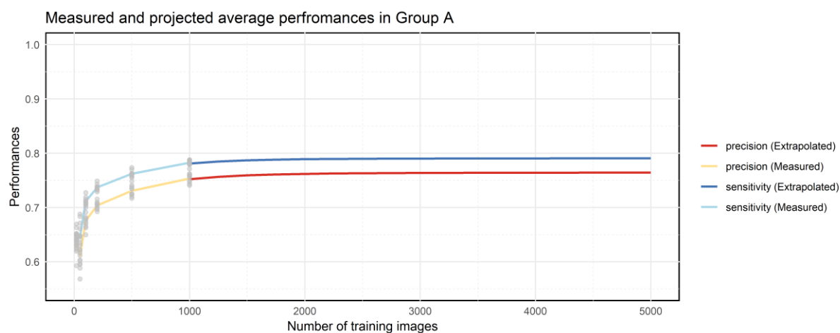
Figure 5-2: Classifier performances (sensitivity and precision) per number of training images measured (20 – 1000) and extrapolated (1000 – 10000). Grey dots show averaged values across all OTUs for each classifier.
