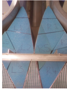
Figure 1: Photograph of the wave flume, showing the high-speed camera for the PIV measurements and the wave probes, looking down-wave towards the beach (a) and up-wave towards the wavemaker (b). Top view photograph of the absorbing beach (c) and a 3D schematic of the beach set-up (d).
