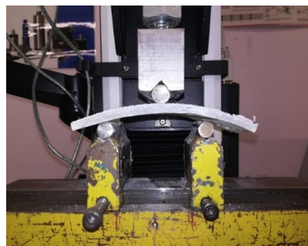
Figure 4: Flexural strength, 3-point bending test set-up.
