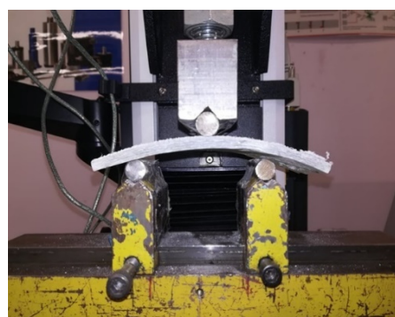
Figure 4: Flexural strength, 3-point bending test set-up.
