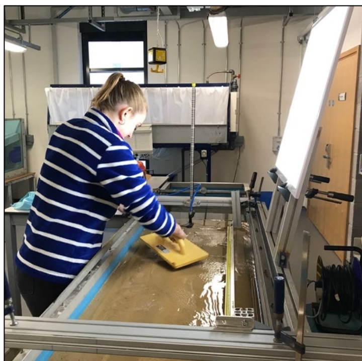
Figure 3: Setup of the sediment bed using a plasterer's float
