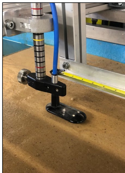
Figure 4: Flow meter suspended over the sediment bed.
