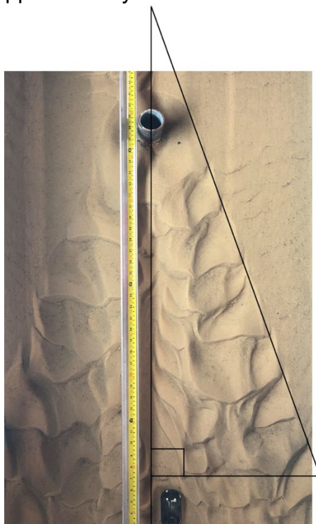
Figure 25: Sketch to determine the angle of propagation of the scour wake from Test 4
