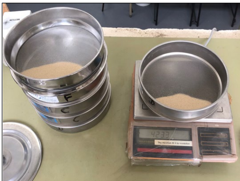
Figure 8: Each sieve was weighed with its contents and the known weights of the sieves were then taken away to determine
