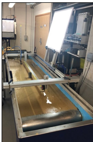
Figure 5: Albion rig setup with LED panel light, suspended tape, flow meter and steel model monopile in place.
