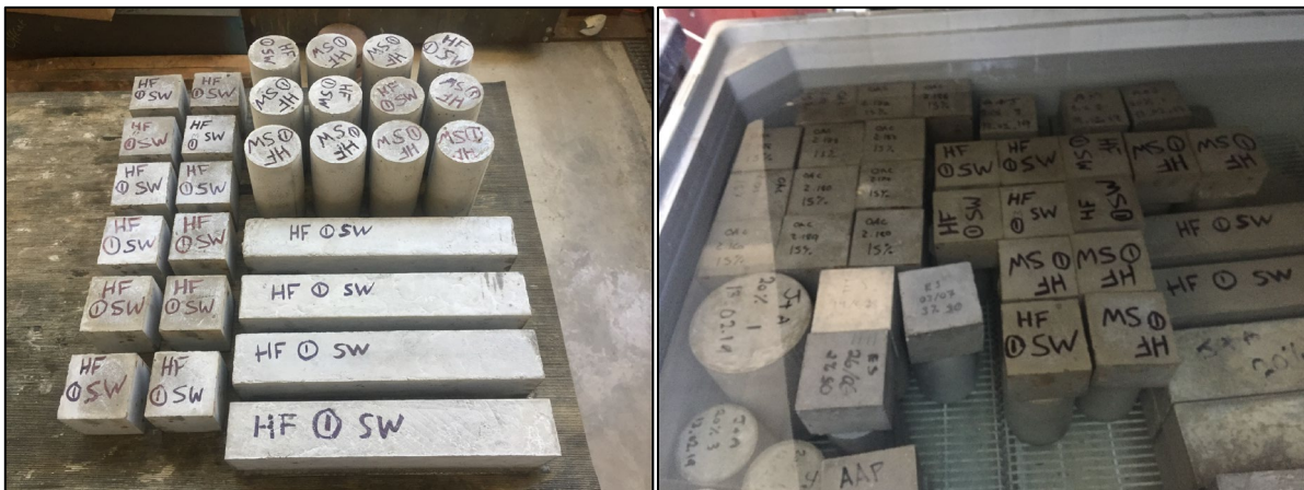
Figure 16: (left) - Samples after un moulding Figure 17: (right) - Samples placed in curing tank
