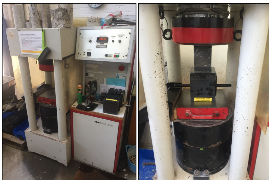
Figure 20: (left) - TONIPACT 3000 hydraulic press Figure 21: (right) - Compressive test on cube
