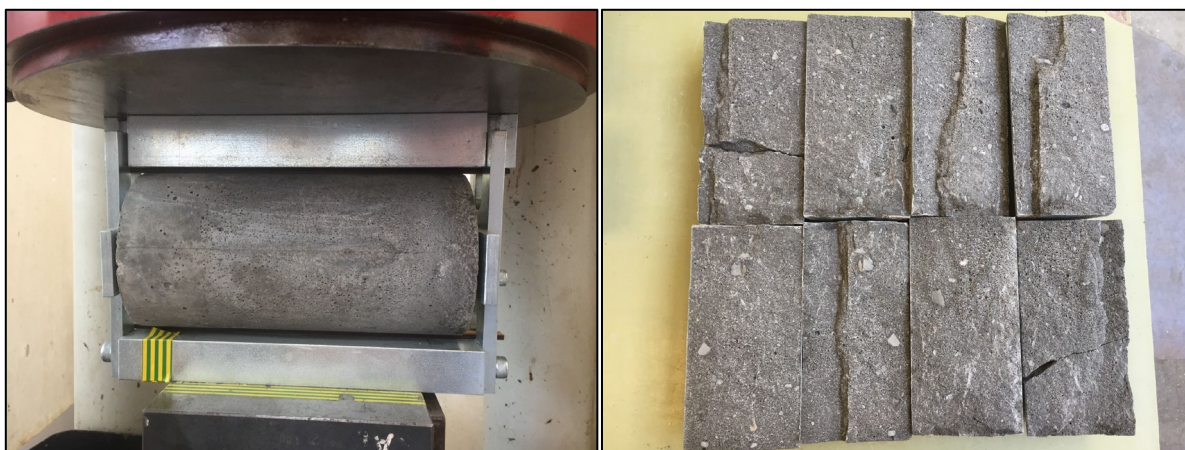
Figure 22: (left) - Tensile test on a cylinder Figure 23: (right) - Broken cylinders after testing
