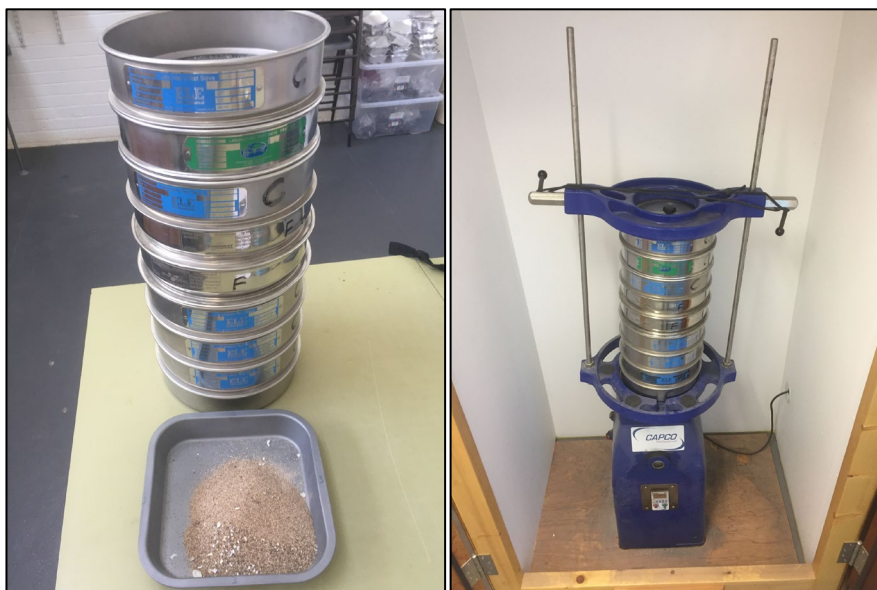
Figure 1: (left) Sieve selection Figure 2: (right) Sieves on the shaker
