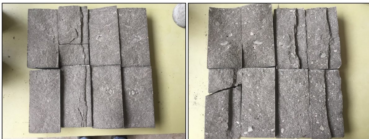
Figure 32: (left) - SW cylinders after testing Figure 33: (right) - FW cylinders after testing
