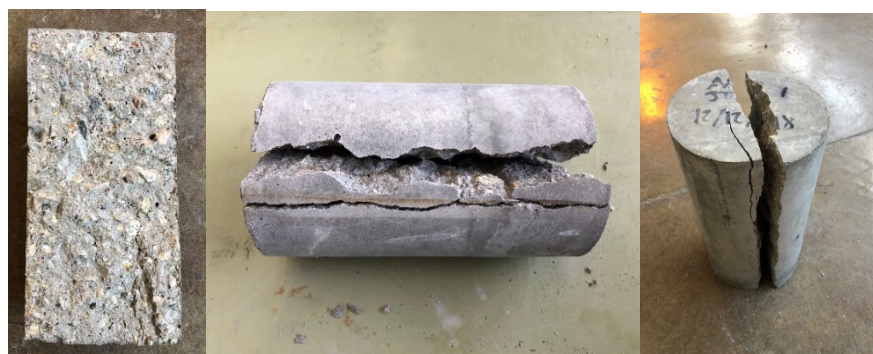
Figure 15: Reference mix sample 1 after splitting tensile failure
