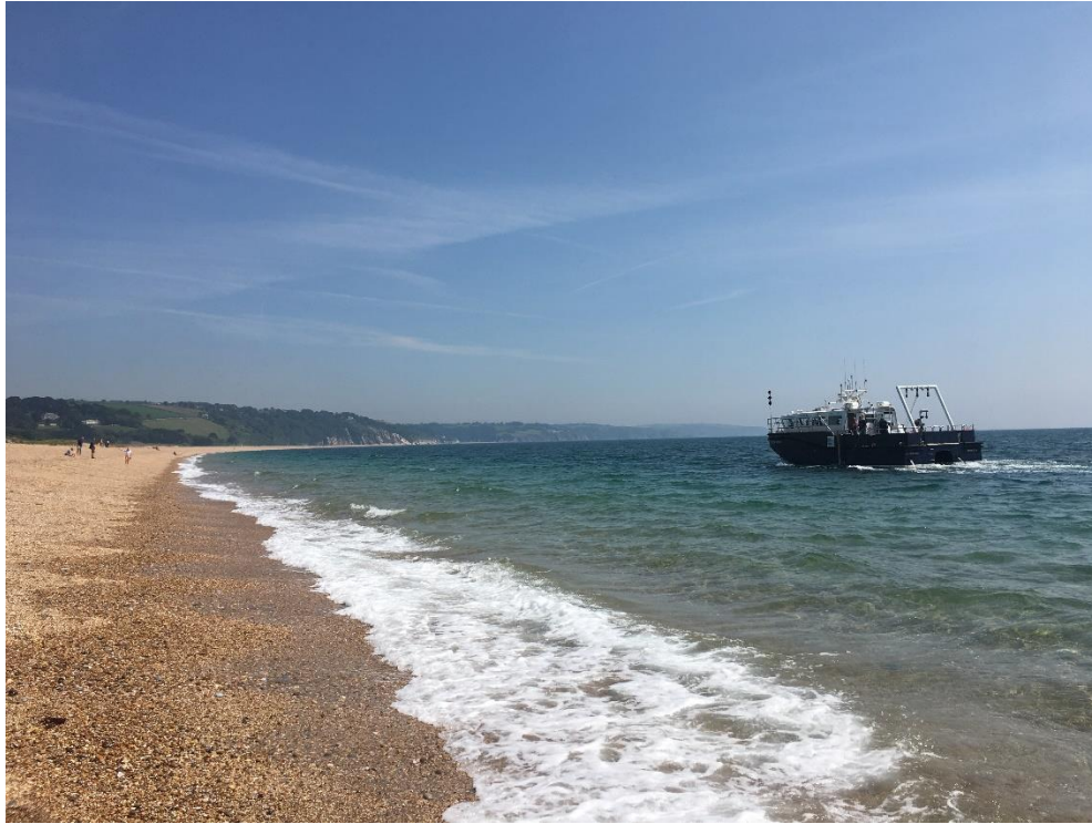
Figure 2.4. The university of Plymouth research vessel, RV Falcon Spirit, conducting a multi-beam bathymetric survey of Start Bay in June 2016, capturing data as close as possible to the intertidal shore face. Copyright Mark Wiggins (2016).
