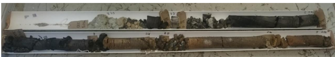
Figure 13: Example of drill core sample no 5 (second yr 2 sample) in two sections: bottom section right to left 0 to 3.75 meters, top section right to left 3.75 to 5.25 m deep.
