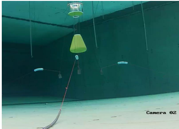
Figure 5: Underwater view of the mooring arrangement of the isolated device setup.
