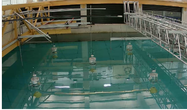
Figure 6: View of the five-device array with mooring configuration C.
