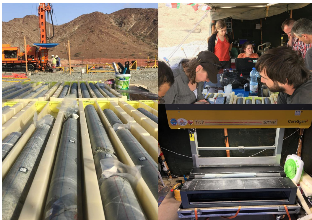
Figure 7.2 – Photographs taken at drill site GT3, showing the drill rig cores in the foreground that are ready to be packed, a group of Phase I scientists describing cores, and the core scanner.
