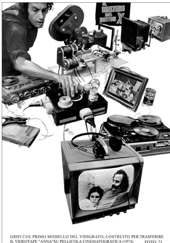
Fig. 9. Alberto Grifi with the first model of 'vidigrafo' [a form of kinescope] that he built to transfer the videotape Anna to film. The picture was published in Video '79 catalogue.
