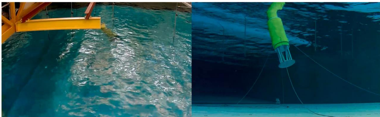
Fig. 18. The CD-OWC model during the survivability test with \square_s = 0.325 m and \square_p = 2.91 s.
