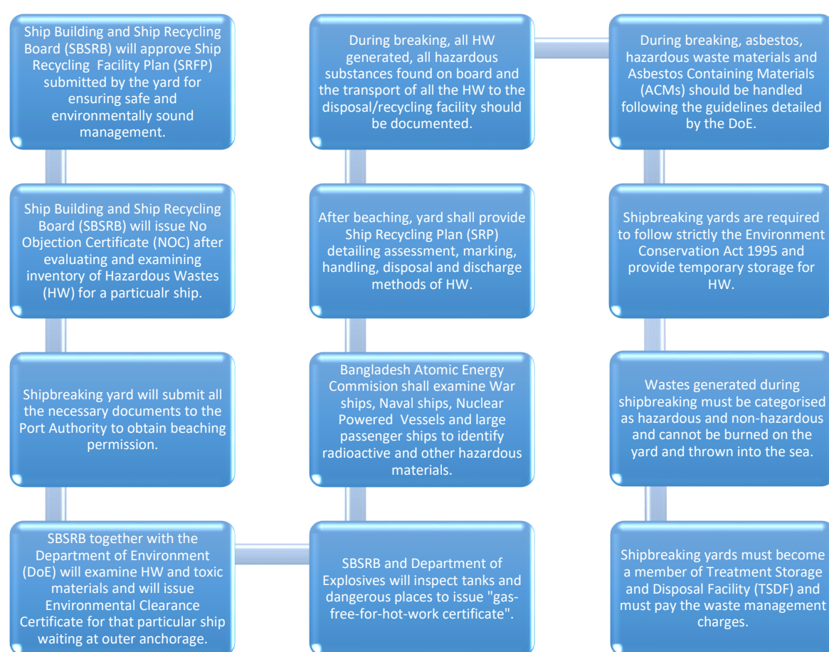
Figure 4: The control and management process of hazardous wastes and materials for a ship planned for breaking in Bangladeshi Shipbreaking Zone (BSZ).
