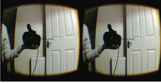
Fig. 7. Radial distortion is added to the input image before it is displayed on the Oculus Rift, to compensate for radial distortion due to the headset’s lenses
