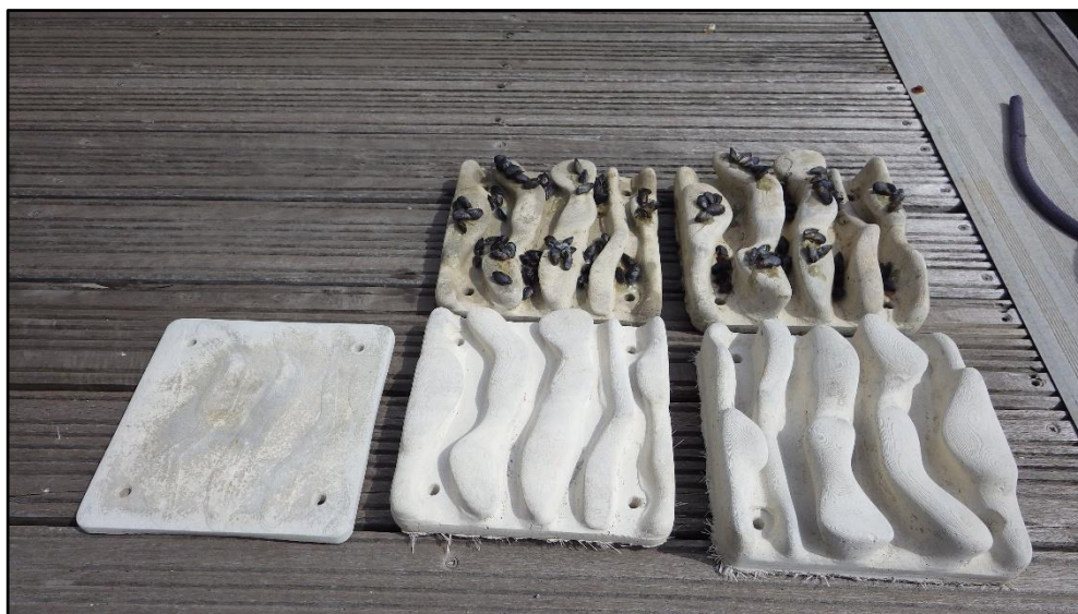
Figure 5-2. Experimental tiles showing (from left to right) the flat, 2.5 cm and 5 cm complexity treatments, with seeded tiles (mussels) shown above.
