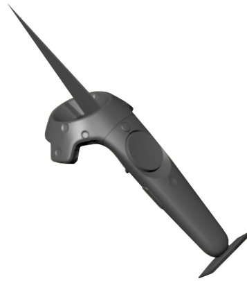
Fig. 3 Visual representation of the manipulated object. The object composed of an edge and a flat part to afford the actions of cutting and crushing.
