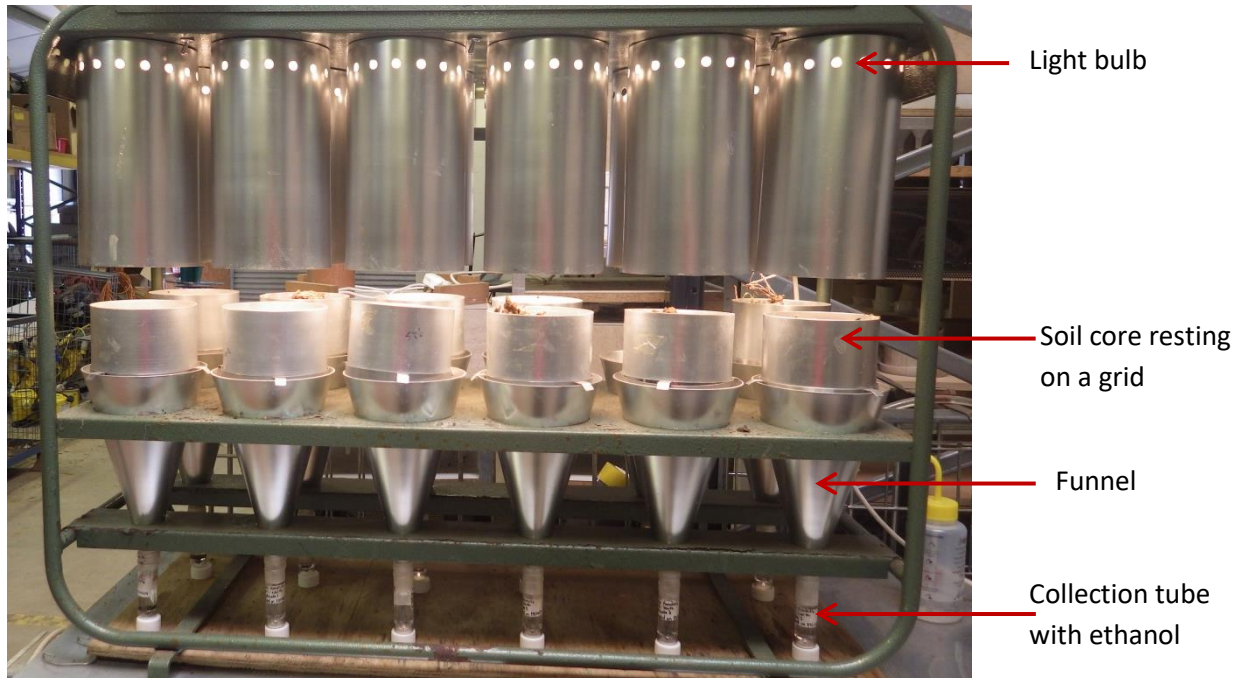
Figure 5.4: Tullgren-funnel system for micro-arthropod extraction from soil samples. The soil core, resting on a mesh, is placed on the top of a funnel. The soil is slowly warmed by a light bulb placed just above, forcing arthropods to move down the soil core to escape warmth, until they fall in the collection tube at the base of the funnel.
