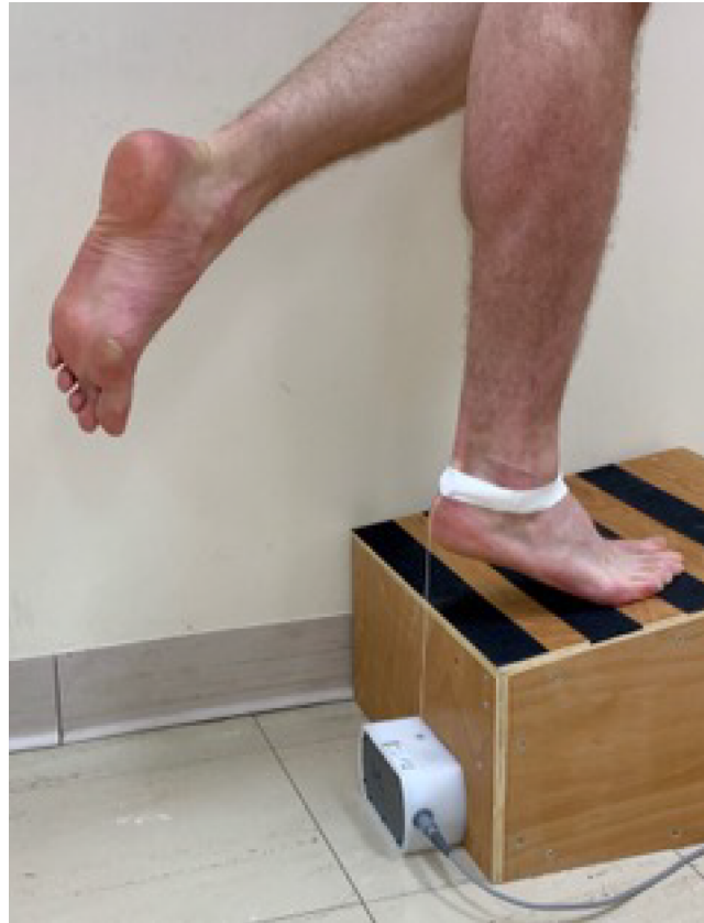
FIGURE 3 A participant performing the HRET. The participant stands on 10° incline box with a cord attached to their heel and connected to a linear encoder, and raises and lowers their heel repeatedly until fatigued.
