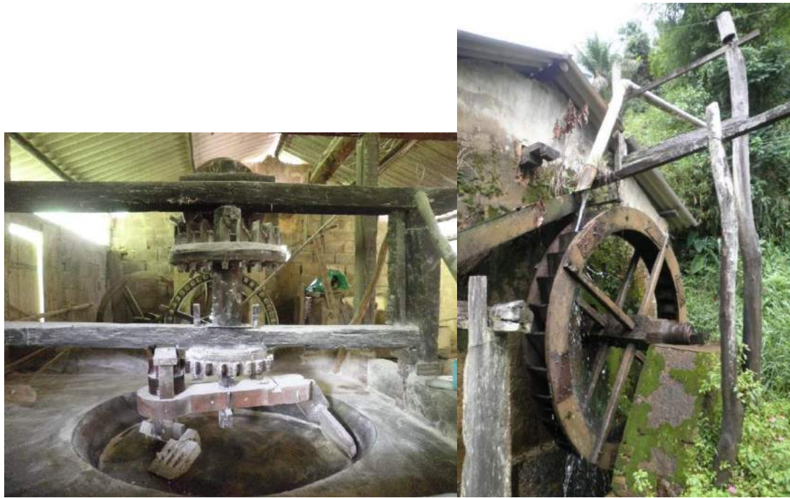
Plate 4.6. Traditional method of preparation of cassava flour in the rural community of Faraó, Cachoeiras de Macacu. The wood structure works through a water wheel. (Source: Author, 2013)
