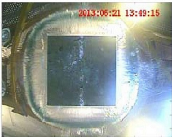
Figure 8.9: Snapshot of view from underneath impact in water for v = 4 m/s (left) Experimental results (right) SPH results.
