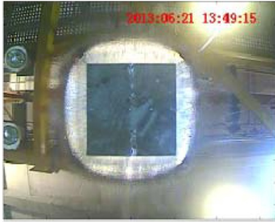
Figure 8.8: Snapshot of view from the bottom dropping flat plate into water during the impact for v = 4 m/s (left) Experimental results (right) SPH results.
