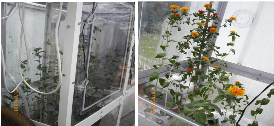
Plate 2. 2. Photograph to illustrate the enclosed \text{CO}_2 chambers used in experiments.
