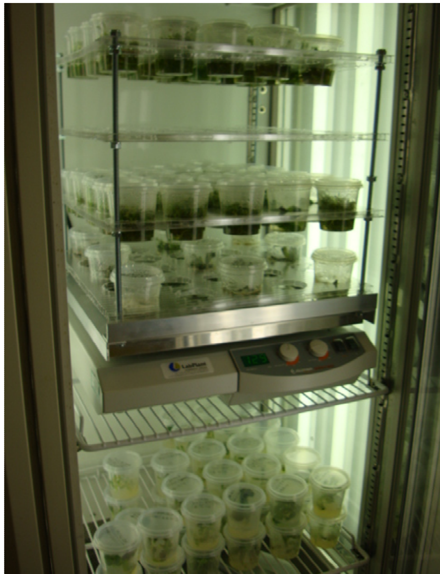
Plate 2.3. Photo to illustrate the growth cabinet (Sanyo plant growth chamber (model MLR-350)) for maintaining the plants after co-cultivation with a bacterial strain. The plants are being grown in shaken liquid media in the upper part of the growth cabinet and in solid media in the lower part.
