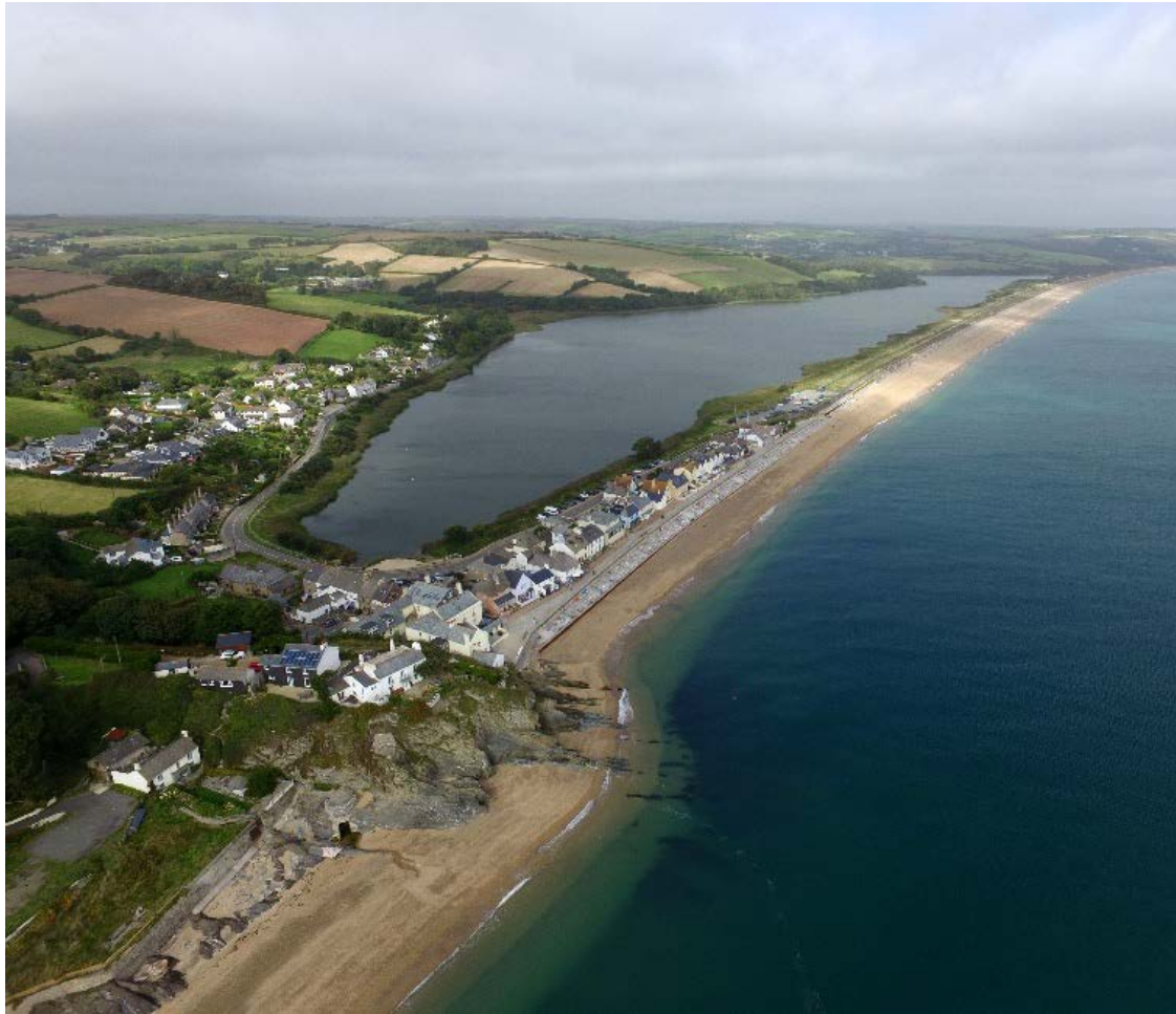
Figure 2 – The village of Torcross, south Devon, England, is situated at the end of a narrow gravel barrier that separates a freshwater lagoon from the sea. An important road runs along the crest of the barrier. The barrier is highly dynamic and erosion resulting from storms and sea-level rise threatens the village and the road. The management policy for the village is hold-the-line, and recent reinforcement of the seawall has undoubtedly contributed to enhanced socio-economic resilience in the short- to medium terms (up to 2050), whilst compromising the natural behaviour of the beach in front to the seawall. The current policy for the road, however, is no active intervention and in case of significant damage to the road it will not be repaired and will thus cease to function. This is likely to have a negative impact on the socio-economic resilience of the region, but it will allow the barrier-lagoon system to function more naturally, thus enhancing ecological and geomorphological resilience.
