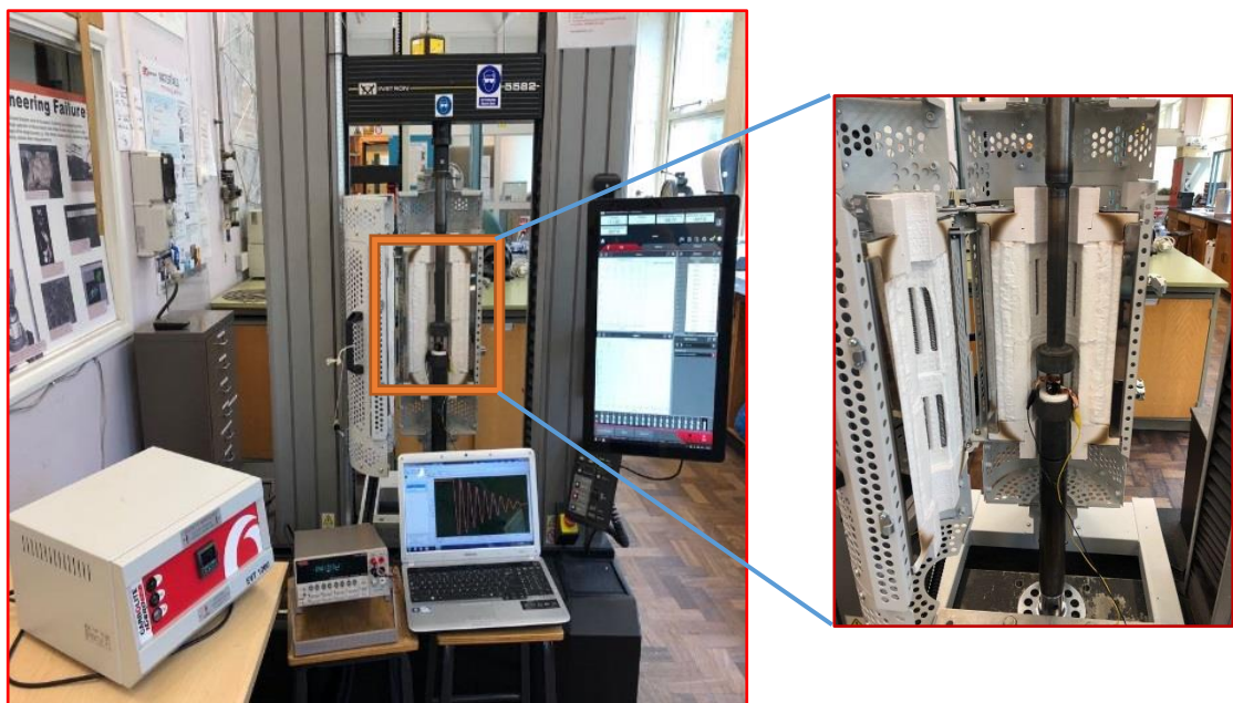
Figure 3.5: Electromechanical test set-up showing the test specimen inside the heating chamber.
