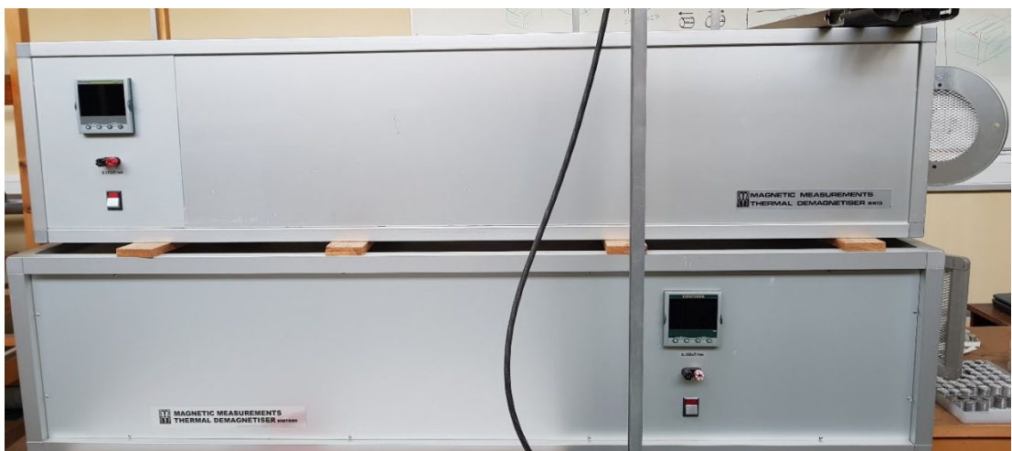
Figure 3.8. Magnetic Measurements Ltd Thermal Demagnetizer – MMTD ovens
