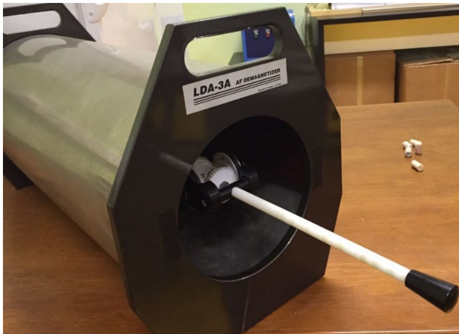
Figure 3.9. AGICO LDA-3 Alternating field demagnetizer
