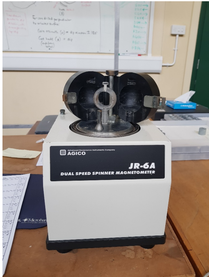
Figure 3.4. JR-6 Dual speed spinner magnetometer
