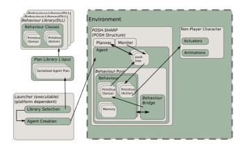
**Figure 1:** The POSH-SHARP architecture once the modules have been integrated into an environment, e.g. the integration with a game engine such as Unity.
