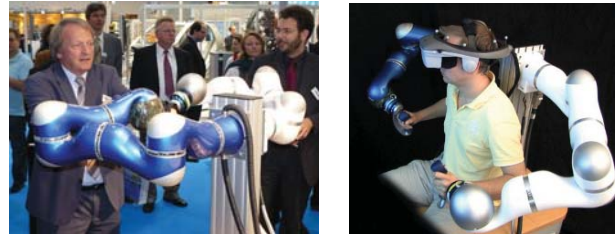
Fig. 1. Two-robot system providing bimanual haptic feedback. (left) Standard configuration, (right) Ergonomic configuration of the bimanual haptic interface.
