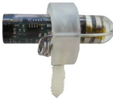
Figure 6.2: DST wired into harness prior to attachment (tag harnesses for DSTs were developed by the MBA behavioural ecology group).
