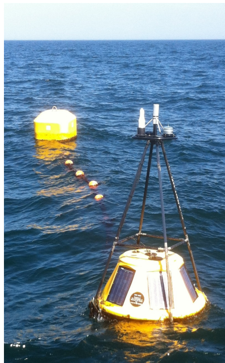
Figure 3.13: Wave buoy deployed at the study site measuring directional wave spectra. Image courtesy of Phil Hosegood (Plymouth University)
