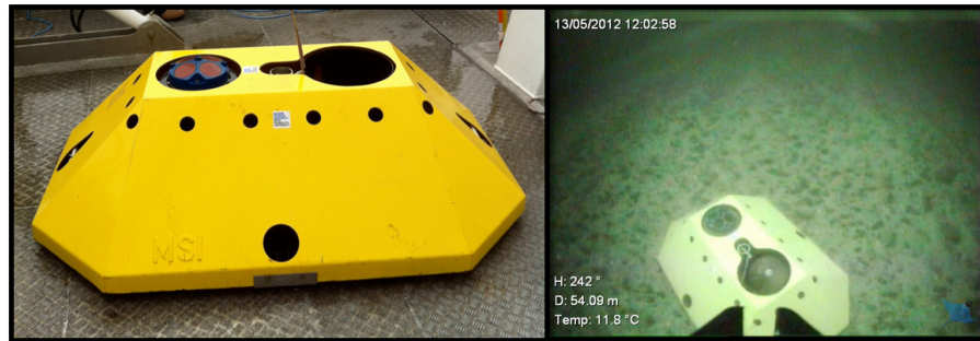
Figure 3.6: Left: Bed-mounted ADCP in a trawl-resistant housing on deck (red circular acoustic transducers in blue casing mounted to the upper face of the yellow housing). Right: Instrument deployed on the seabed at the study site in May 2012. The ADCP was recovered using a positively buoyant recovery line stored within the housing and released via an acoustic release mechanism.
