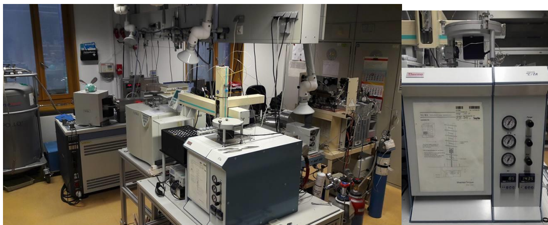
Figure II-10: Thermo-Finnigan High Temperature Conversion Elemental Analyser coupled with a continuous flow mass spectrometer at the Geowissenschaften, Goethe Universitat, Frankfurt, Germany.
