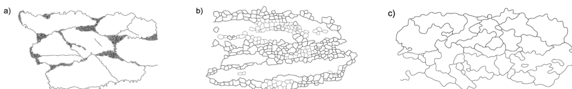
Figure II-5: Characteristic microstructures of the three dynamic recrystallization mechanisms of quartz shown at the same relative scale. (a) Bulging recrystallization (low temperature): bulges and recrystallized quartz grains are present along grain boundaries and to a lesser extent along micro cracks. (b) Sub grain rotation recrystallization (intermediate temperature): core and mantle structures of porphyroclastic ribbon grains and recrystallized sub grains. Polygonization by progressive sub grain rotation can completely consume the ribbon grains. (c) Grain boundary migration recrystallization (high temperature): irregular grain shapes and grain sizes; grain boundaries consists of interfingering sutures (Stipp et al., 2002).
