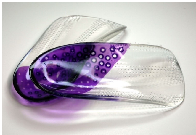
Figure 6.2 The handmade prototypes used for proof of concept testing with the cones visible in the medial arch area
