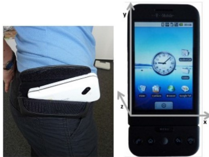
Figure 3-5: Phone attached to the subject and the three axes in which acceleration measured (Derawi et al. 2010)
