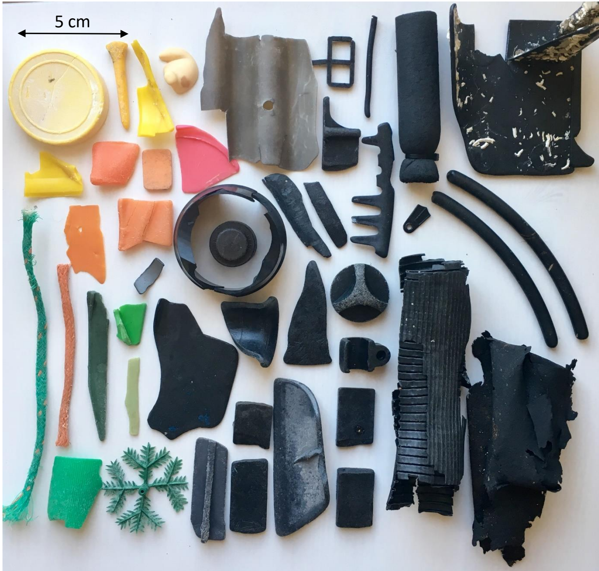
223 Figure 2: Examples of beached plastics from south west England that were non-compliant or 224 potentially non-compliant with respect to RoHS regulations.
