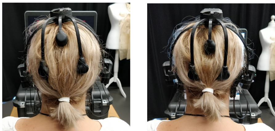
(a) Electrode positions for placement I . (b) Electrode positions for placement II .
