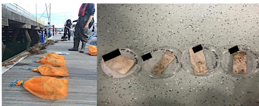
Figure 4.1. Left – Whole baby-wipes which have been sewn into mesh pouches and placed in an orange high-density polyethylene bag before deployment into the marine environment (Queen Anne’s Battery Marina; Plymouth). Right – Extracted baby-wipes after 1 week exposure in the marine environment. The brand names on the petri dishes have been removed.
