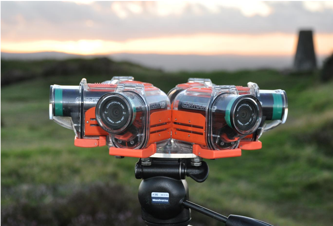
Figure 17 360-degree rig with six separate HD Contour cameras. Image by Karol Kwiatek.
