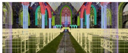
Figure 9 3D model overlaid with panoramic picture.
