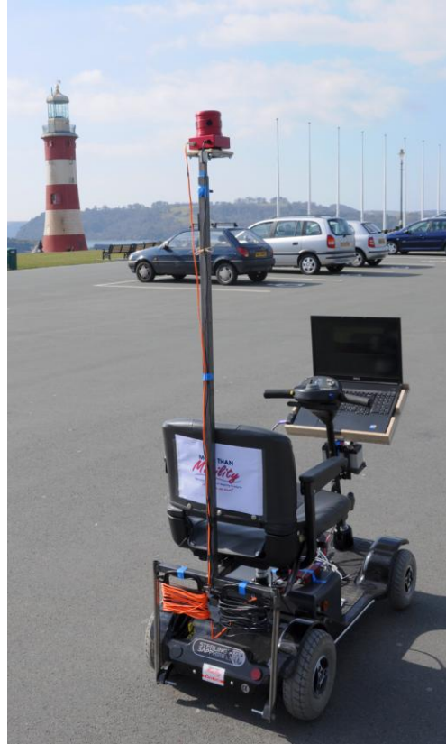
Figure 71 A motorised scooter adjusted to be used with Ladybug@2 camera and a laptop (July 2010). Image by Karol Kwiatek
