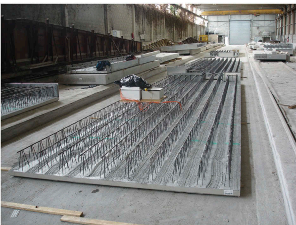
Figure 4. Lattice girder flat slab with embedded sensors and data acquisition system.
