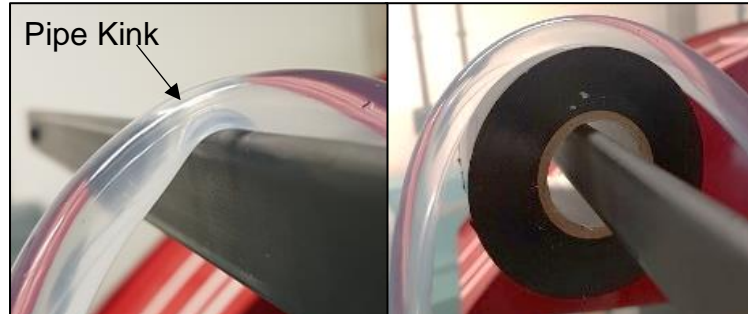
Figure 5: Tape roll to prevent pipe kinking.
