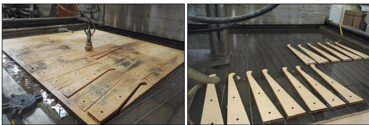
Figure 3: Seawall offcuts produced from an 8m x 4m sheet of 12mm plywood
