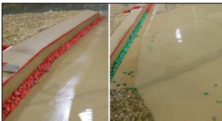
Figure 32: HR Wallingford physical model experiment of the Hinkley Point C seawall showing rock damage
