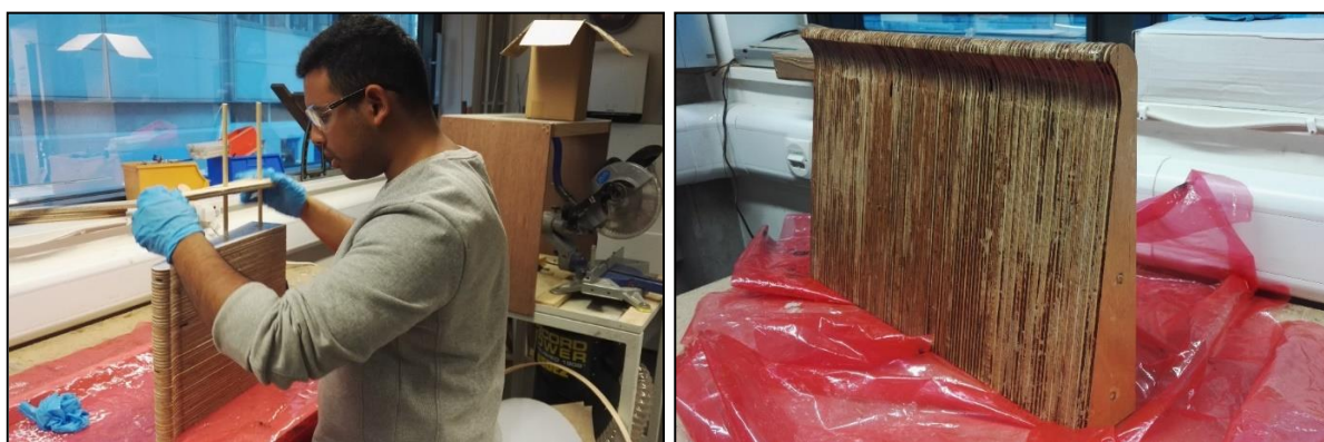
Figure 4: Gluing the offcuts and aligning them with the use of dowels
