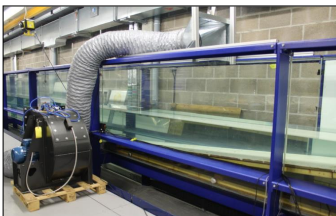
Figure 11: Wind generator set up
