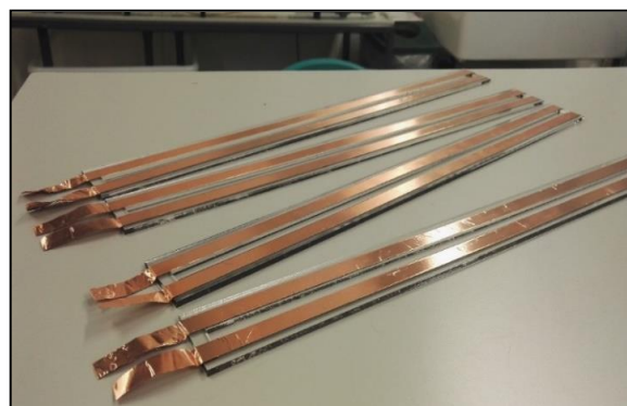
Figure 8: Wave gauges with copper tape attached
