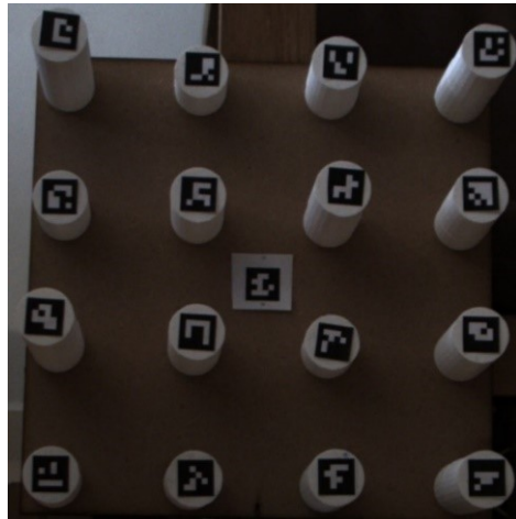
Figure 6-7. A template for in-depth measurement with 16 targets at different heights.
