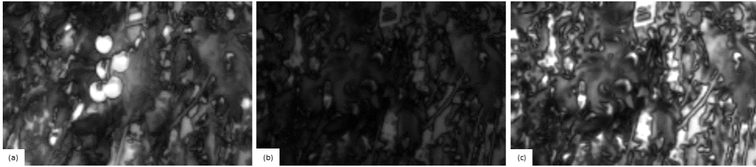
Figure 7-9: Conspicuity maps of three input feature map. (a) colour, (b) intensity, and (c) orientation.
