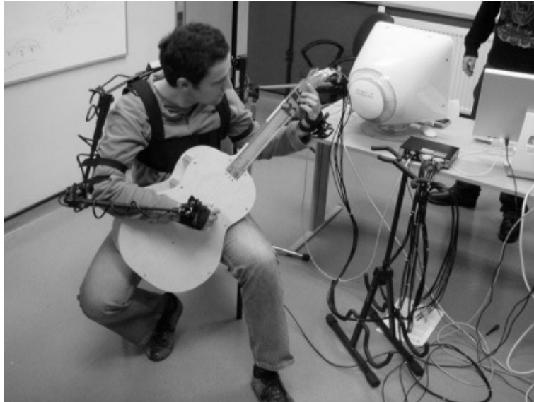
Figure 5 : Subject trying the force measuring apparatus. Setup composed of a Gypsy6 exo-skeleton and FoGu – a custom made guitar that records the coordinate finger's force production.
