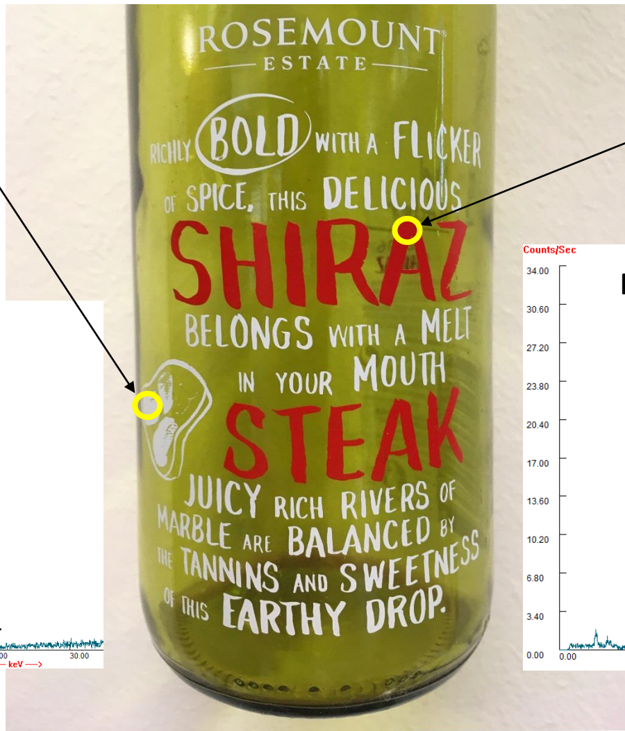
Figure 1: A UVAG-coloured and enamelled wine bottle with spectra arising from the XRF measurements (handheld and 3-mm collimation) of the red and white decorated areas indicated by yellow circles. Note the presence of Se in the red enamelled area indicative of the use of cadmium sulphoselenide. Also shown are Cd, Pb and Cr concentrations ( \pm 2 counting errors) over both measurement areas.
