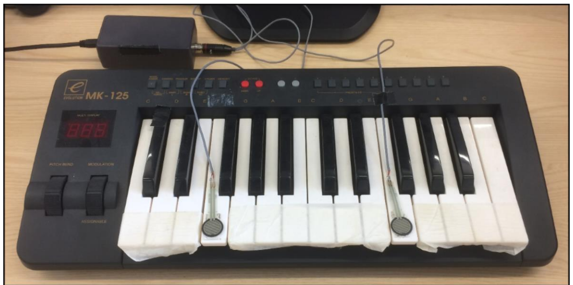
Figure 13. The custom hardware developed for the pressure-based version of the intention insertion task in Experiment 4. This interface consisted of a standard musical keyboard and two force-sensitive resistors, or “pressure pads” to record the pressure exerted by each of the participant’s fingers for the duration of the experiment. The keys facilitated a good range of movement and the spacing between the two active keys was similar to the keyboard-based intention insertion task used in Chapter 2.
