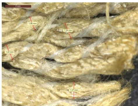
Figure D.10: 2M NaOH 72h flax treatment measurement 7
