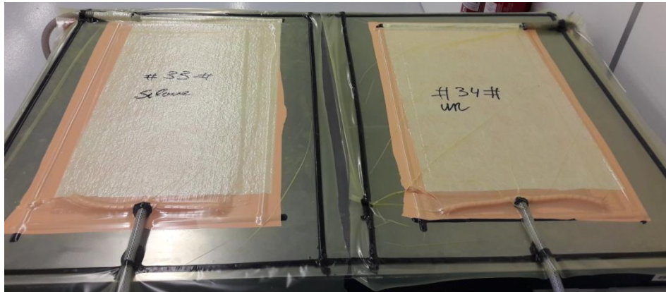
Figure 7.19: manufacturing process of laminates 33 and 34
