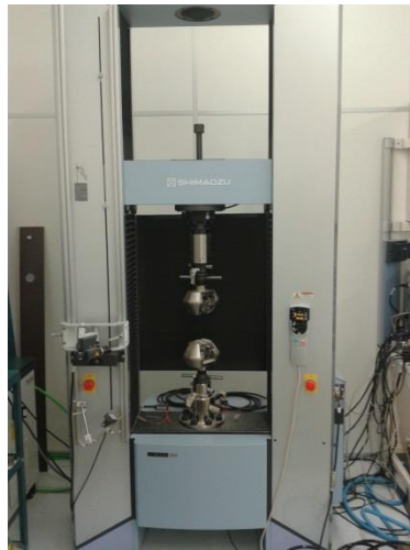
Figure 7.9: Shimadzu AG-X PLUS 250kN Universal testing machine
