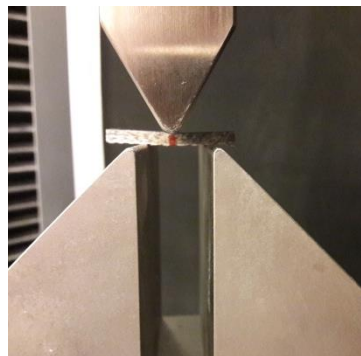
Figure 7.23: Short-beam test sample
