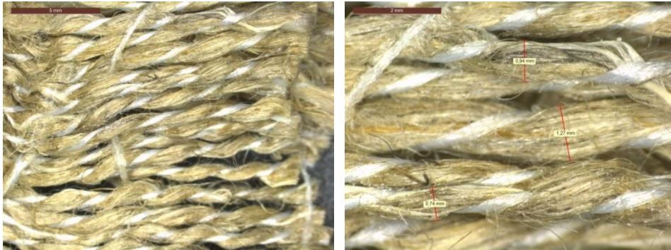
Figure D.1: Untreated flax fabric panoramic picture (left) and measurement 1(right)
