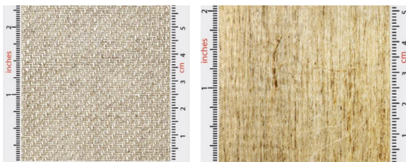
Figure 7.2: Flax-ply woven and UD fabric (Courtesy of Easy Composites)
