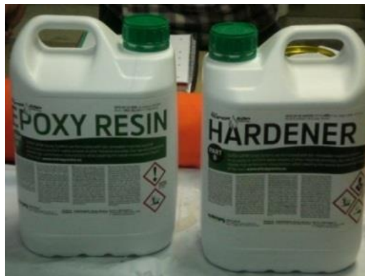
Figure 7.4: Supersap CLR/CLX system used for the panel production (Courtesy of 5TX surf)
