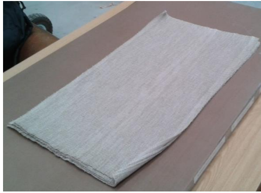
Figure 7.3: Flax-ply woven and UD fabric
