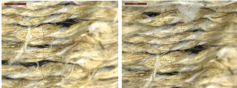
Figure D.8: 2M NaOH 72h flax treatment measurement 3(left) and 4 (right)
