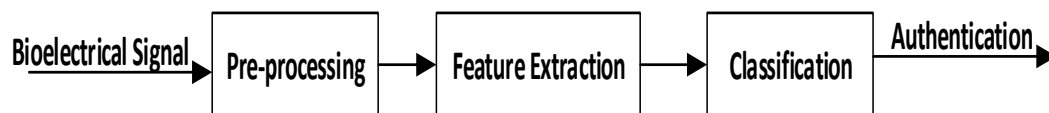
Figure 3. Error! No text of specified style in document..4: Block diagram for processing bioelectrical signal system for authentication.
